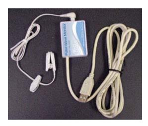
The PW-1000 unit has a standard USB cable with a flat USB connector.
